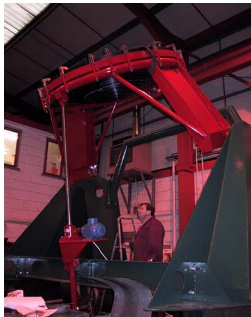
Figure 1: One of the L-band lenses and drive systems now installed on E-systems antennas
