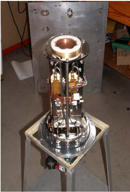
Figure 2: One of the new e -MERLIN C-band receivers under assembly in the cryogenic laboratories at Jodrell Bank
