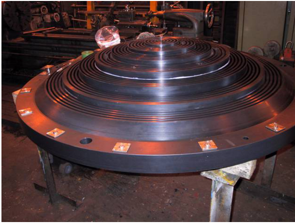
Figure 3: a) The L-Band lens being fabricated in the SHAL factory, Chesterfield. b) Installation at Pickmere.
