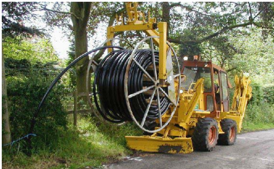
Figure 33: Moleploughing equipment and the cable duct for the e-MERLIN optical fibre network.
