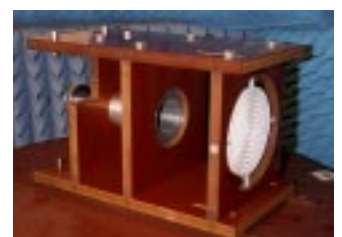
Above: Scaled L-Band horn and lens.
