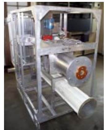
Above: Building the new Defford dual band focus box.
