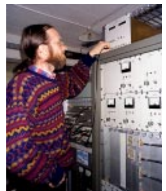
Above: A VLBI technician installs the Mk IV recording upgrade.
